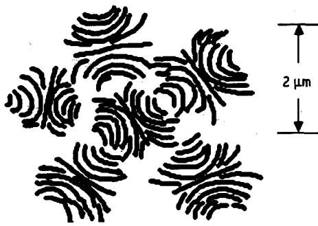
Figure 4 A schematic of the sheaflike structure in 450G PEEK.
